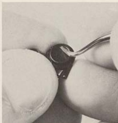
Fig. 13. Before mounting an instrument face, carve a shallow groove in the bezel to which it will be attached.
