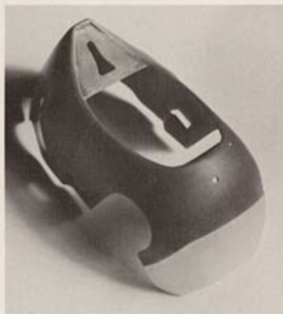
Fig. 15. All parts of the fairing must be smooth before any paint is applied. The plastic windshield on the Suzuki fairing is milky at this stage but will be polished until it is perfectly clear.
