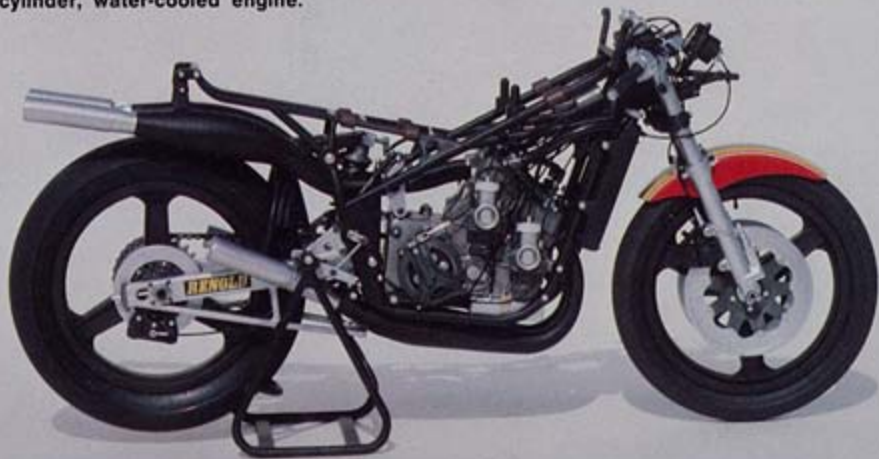
Fig. 1. Removing the fairing and gas tank reveals the superdetailed 4-cylinder, water-cooled engine.
