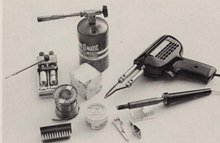
Fig. 1. The author uses these tools and materials for soldering brass and steel parts. Clockwise from top: propane torch, soldering gun, soldering iron, heat sinks, Nokorode brand paste flux, brass-bristled brush for cleaning tips, 50/50 solid lead-tin solder, sal ammoniac block, and Microflame oxygen torch.
