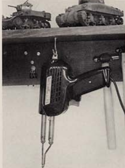
Fig. 2. Paul's favorite soldering tool is this high-wattage gun. He fabricated the metal bracket on the back of the gun so he could hang it at his workbench.
