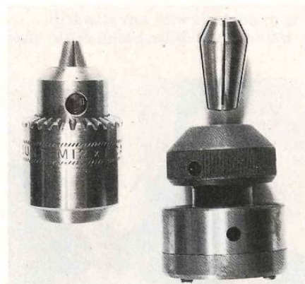
Fig. 1. A drill chuck (left) and a collet chuck. The disadvantage of the collet chuck is that it requires a different collet (the piece shown above the chuck) for each drill size or tool shank.
