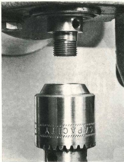
Figs. 2 and 3. (Left) a drill chuck with a socket that fits on a tapered shaft, and (right) another chuck that screws onto a threaded arbor. Both types are common.
